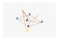
Figure 1.27: First flexible mode at 692Hz
