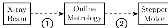
Figure 3.1: Schematic of the calibration procedure: the stepper motors are calibrated from the online metrology (i.e. the interferometers) which is itself calibrated using the x-ray beam
