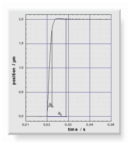
Response behavior of the P-562.3CD: Step-and-settle in less than 10 ms in X, Y, and Z.
