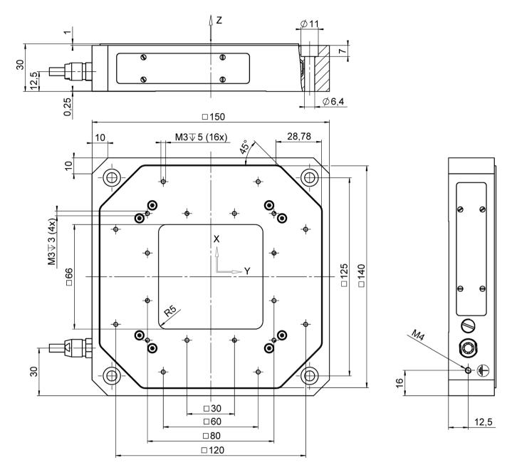
P-56x.3CD and P-56x.3CL, dimensions in mm
